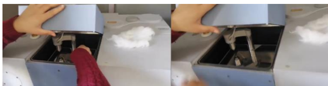
Figure 2 Identify FTIR spectra of MAC at the Egyptian National Research Centre central lab.
