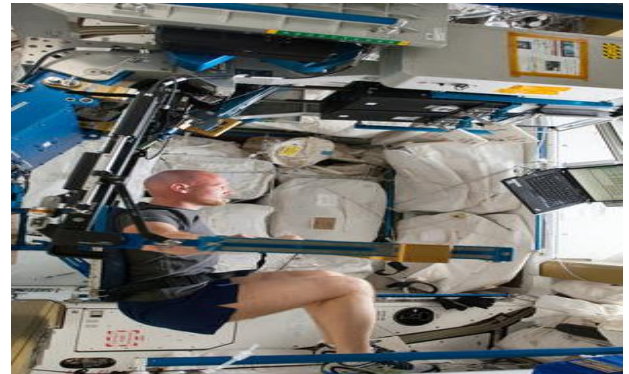
Figure 2: ESA (European Space Agency) astronaut Alexander Gerst gets a workout on the Advanced Resistive Exercise Device (ARED) in the Tranquility node of the International Space Station.
